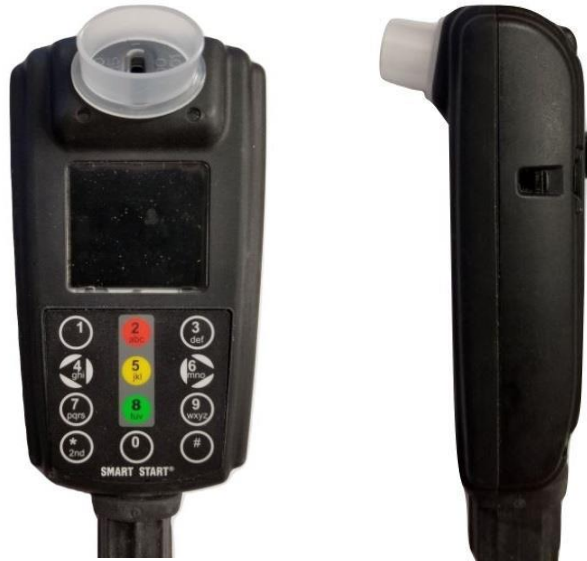
Figure 4 Properly Inserted Mouthpiece
