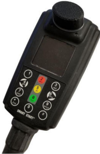
Figure 6 Head Unit with Mouthpiece Cover attached
