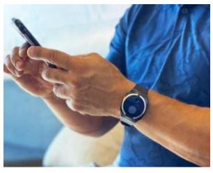
"Other devices 'sniff' the skin using a pump and a breath alcohol fuel cell," he said. "ORBIS continuously monitors using a specially designed transdermal sensor. This patent pending technology allows us to offer unprecedented accuracy in a design that is the most discreet and smallest in the market."
